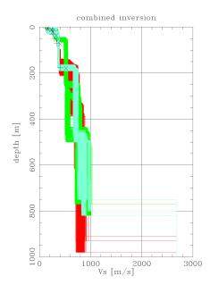
Figure 3.15: Velocity models with acceptable misfit found for Martigny (red), Saillon (cyan) and Vetroz (green) with all valley parameterisations. The black symbols show shear-wave velocities obtained with other methods.
